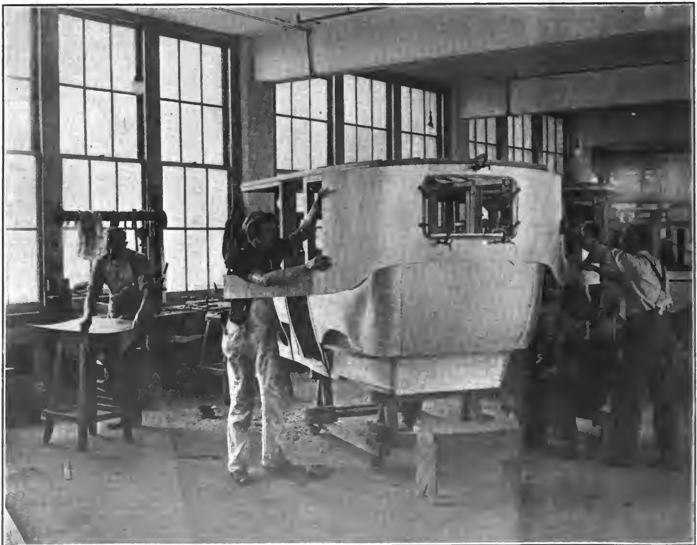
BODY MAKING ILLUSTRATED—TAKEN AT PACKARD PLANT, DEPICTING METHOD OF LAYING ON ALUMINUM SHEETS
